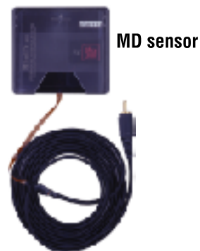
Connecting cord of MD sensor and DVD-RAM
